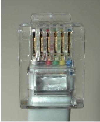
Insert the conductors into the modular connector so that the white wire is on the left with the modular connector positioned for insertion into the autoguider socket on the LX200 panel (locking tab down). After crimping, the end of the cable should look like the image to the left:
