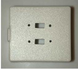
Select suitable locations for the two slide switches; they must be installed away from the edges of the cover so that the switch terminals and mounting screws do not come in contact with the modular jack terminals. Drill holes for the mounting screws and cut the openings for the switches as shown in the image to the left:
