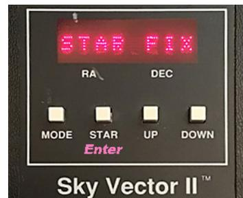
A list of alignment stars appears, scroll with **Up/Down** to first desired star, for example Vega (don't press any button), then move scope so as to get first desired star centered in your eyepiece, press **Enter**. The alignment star list reappears automatically.
