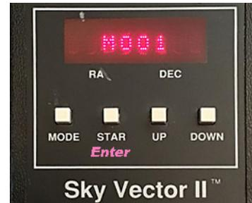
Additionally, after setting the catalog number, pressing **Enter** once will display its RA/DEC location, a second press will give a brief description of the object. Then...
