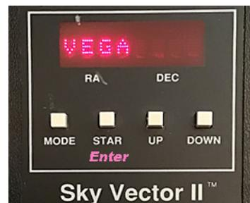
Press **Mode** to go to **SetUp/Date** (two digits for month/day/year) to verify it is correct and, if necessary, adjust to today's date by changing numerical choice
